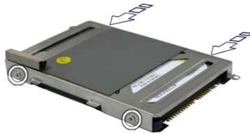
Fig. 16 Removing the hard disk drive brackets
